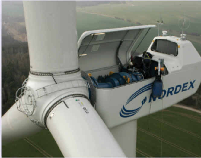
Figure 26.1: This giant wind turbine uses electromagnetic induction to produce electricity. Look for the two engineers at work. (You can identify them by their white helmets.) This gives you an idea of the size of the generator.
