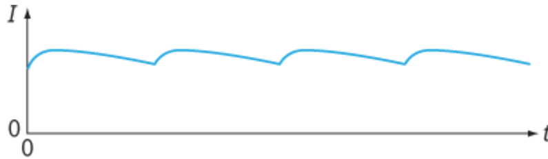
Figure 27.17: A smoothed, rectified current. For Question 14.
