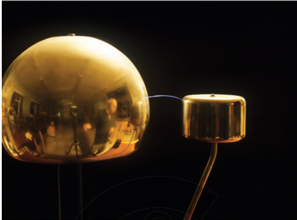
Figure 21.13: A Van de Graaff generator produces voltages sufficient to cause sparks in air.
