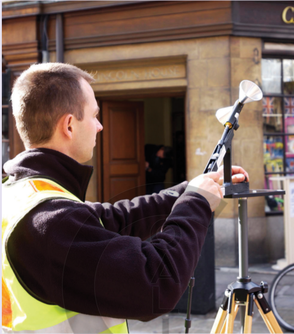
Figure 22.1: Mobile phone masts produce weak electric fields – this scientist is using a small antenna to detect and measure the field of a nearby mast to ensure that it is within safe limits.
