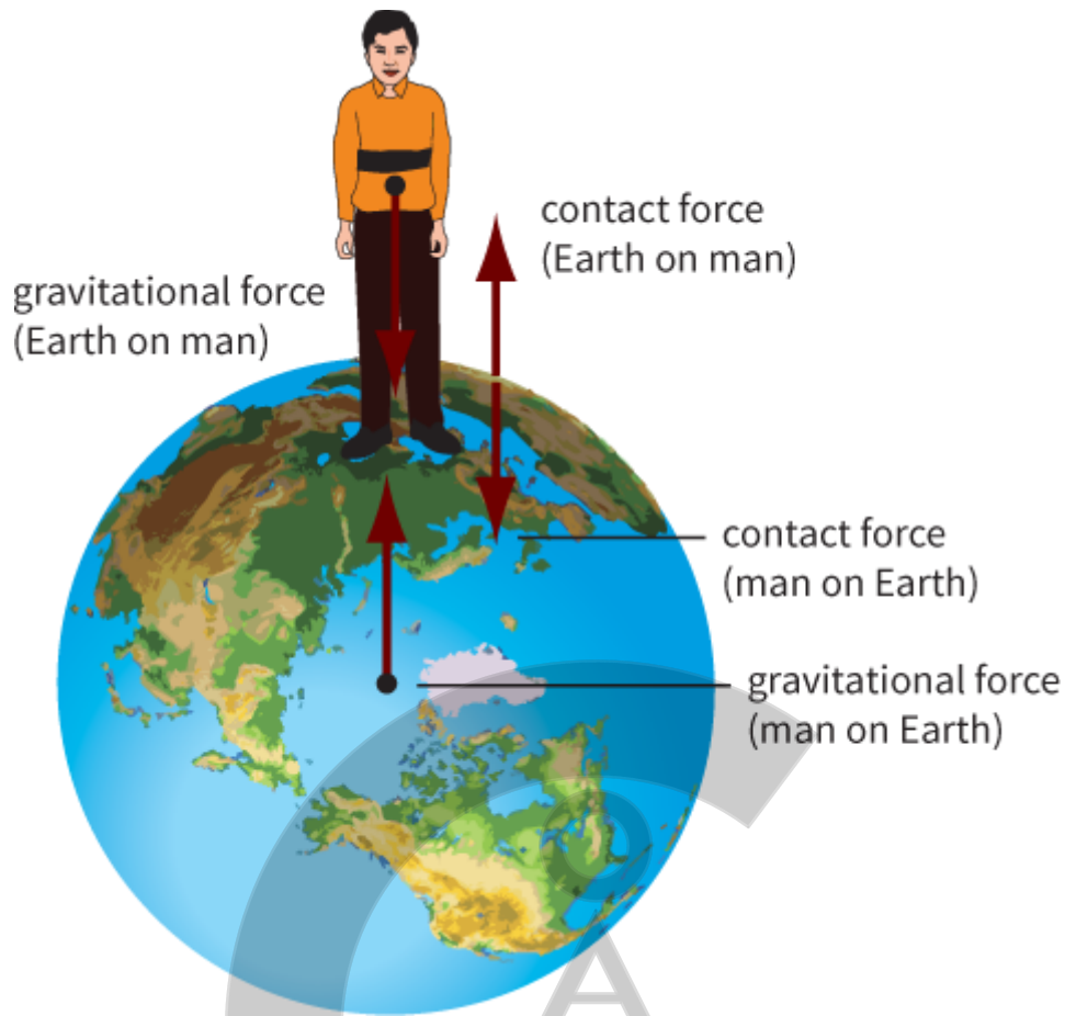
Figure 3.16: For each of the forces that the Earth exerts on you, an equal and opposite force acts on the Earth.
