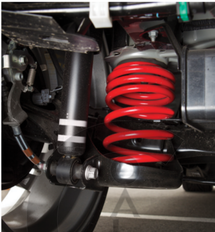
Figure 18.28: The springs and shock absorbers in a car suspension system form a damped system.
