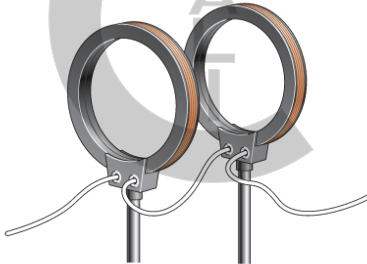
Figure 25.10: A pair of Helmholtz coils is used to give a uniform magnetic field.
