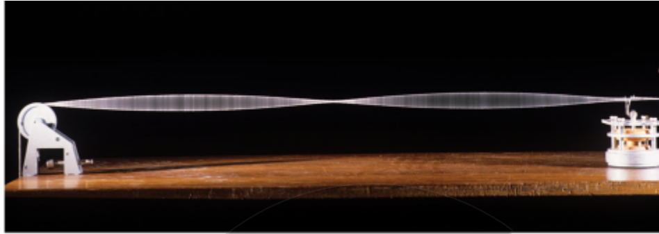
Figure 14.7: When a stationary wave is established, one half of the string moves upwards as the other half moves downwards. In this photograph, the string is moving too fast to observe the effect.
